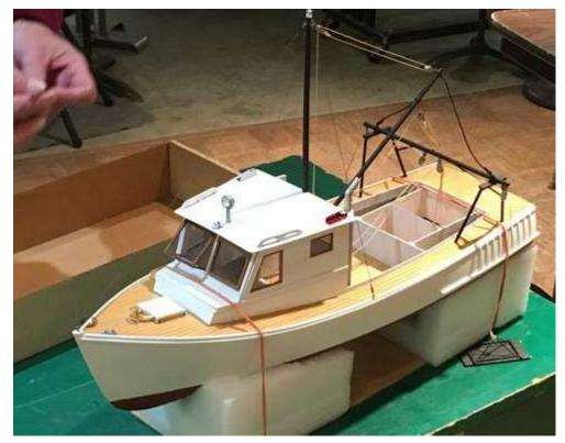
You have to stare at this one for a bit to take in all the details that allow the real boat to spread nets for the catch. Note the boom to lift the nets and the planing boards to spread the nets. In addition the size of the kit made access to the electrics below deck a bit tight so the cabin is fabricated to be completely removable in sections. Tim has
